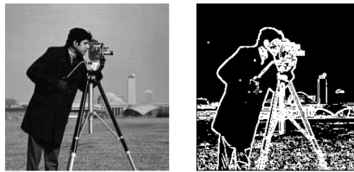
(a)Original Grayimage (b) edge detected output Figure.13 Simulation result for canny edge detection
